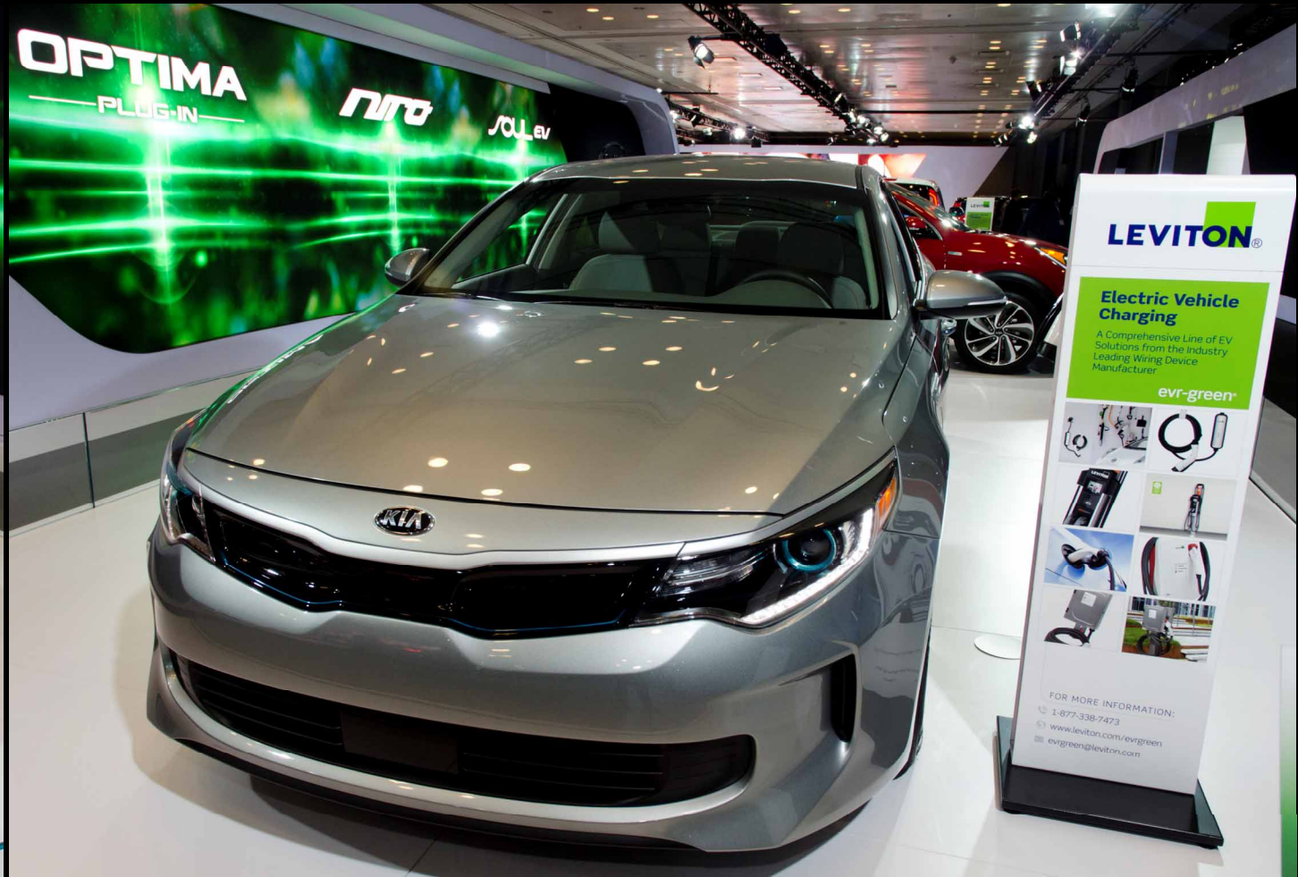
2017 KIA Optima Plug-in Type: Full Hybrid System Mileage: 99 MPGe Range: 27 miles (battery-only) Cost: $27,700.00
